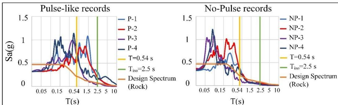
Figure 3. Spectral accelerations of the scaled records on Rock (class A), log scale.
