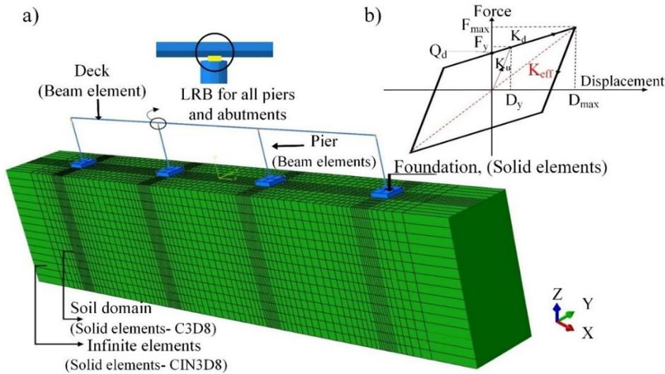
Figure 2. The global model of the isolated bridge and soil, and the bilinear force-displacement relation of the Seismic Isolation System (SIS) (a) Isolated bridge model and soil (b) bilinear force-displacement behaviour of SIS.
