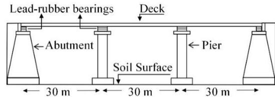
Figure 1. General elevation of the isolated bridge.
