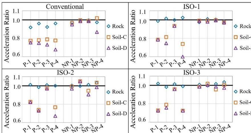
Figure 5. Acceleration ratio (SSI/Fixed-base).
