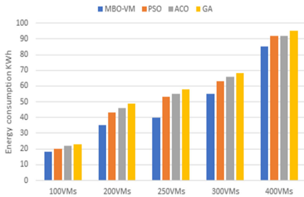
Fig. 4 Average power consumption of all active PMs of HP ProLiant ML110 G4 type
