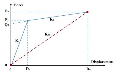
Figure 3. Idealized non-linear force-displacement curve for HDRBs [22].
