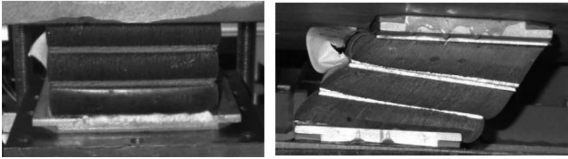
FIGURE 3 Deformed bearing under a compression load of 19 kN (left) and a combined compression load and shear displacement (right) during the experiment. 44
